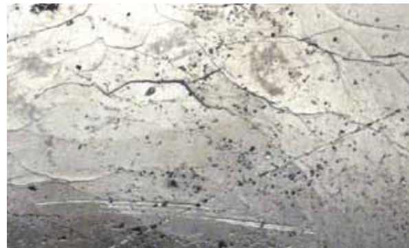
Stress Corrosion Cracking Stainless Steel in Seawater Environment
