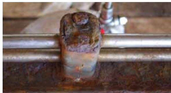
Crevice corrosion between the tube/tube trap interface.
